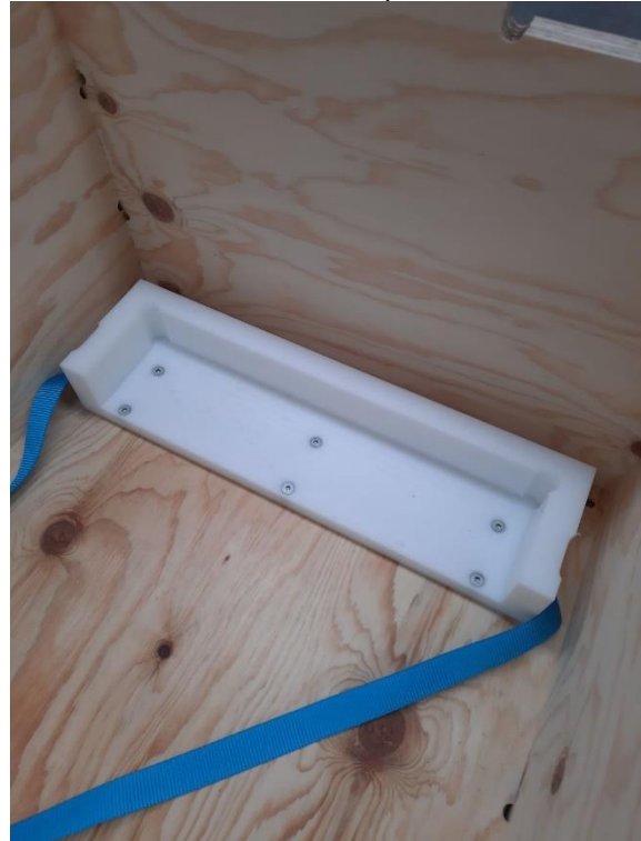
Plastic textile strap under plastic profile
